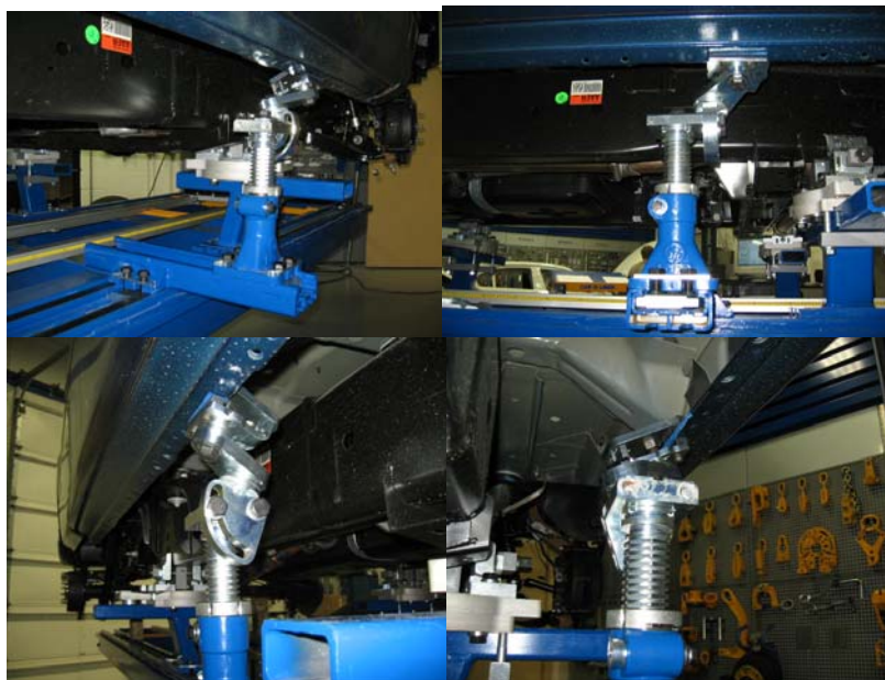
Universal Clamping to Pinchweld Area Using EVO
