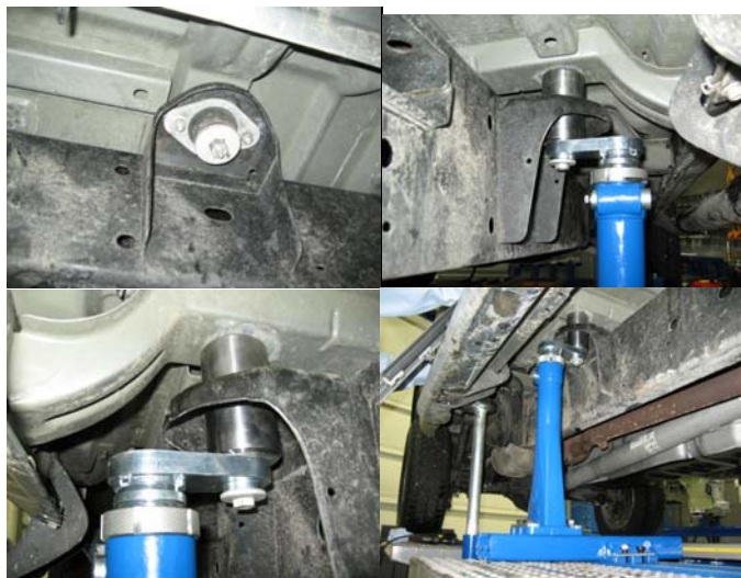
NOTE: MOUNT AREA AND BUSHING PLACEMENT
